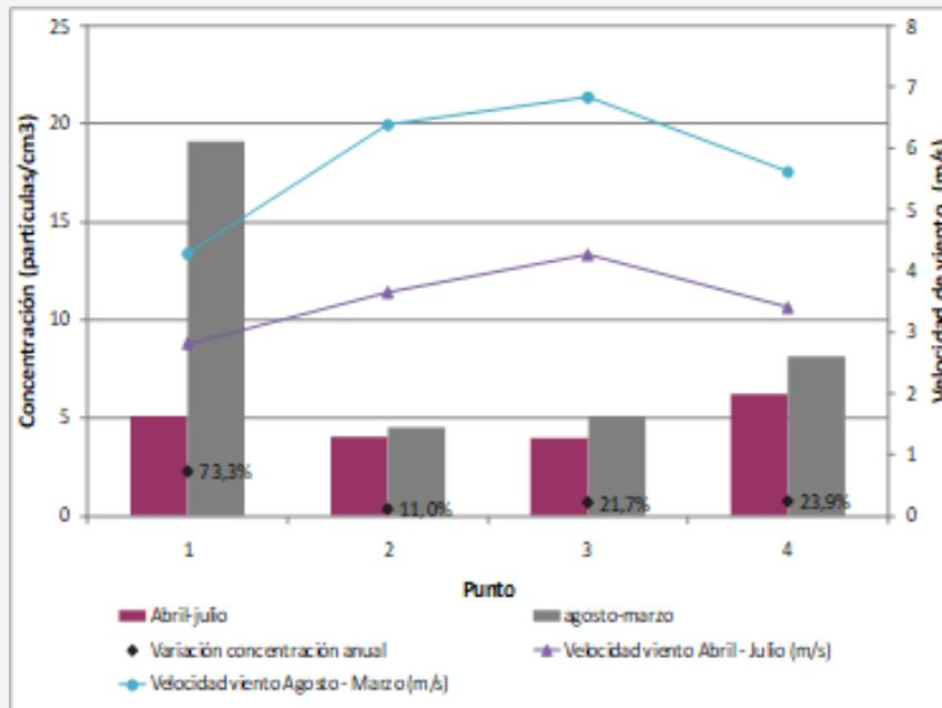
Figure 6: Averages of wind speed and concentration of PM10 and its variation in monitoring stations.
