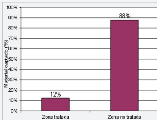
**Figure 4:** Distribution of the total material collected in the dust collectors, location in the area treated with dust suppressant and untreated areas.
