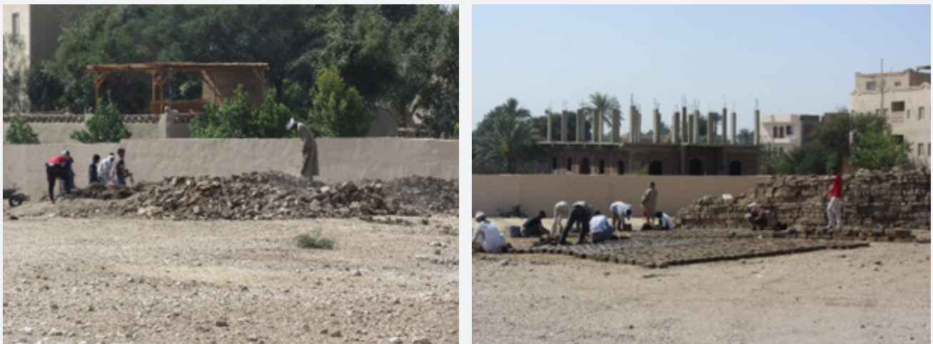
Figure 2: Recycling of mud brick scrap (left) to make new mud brick (right).
