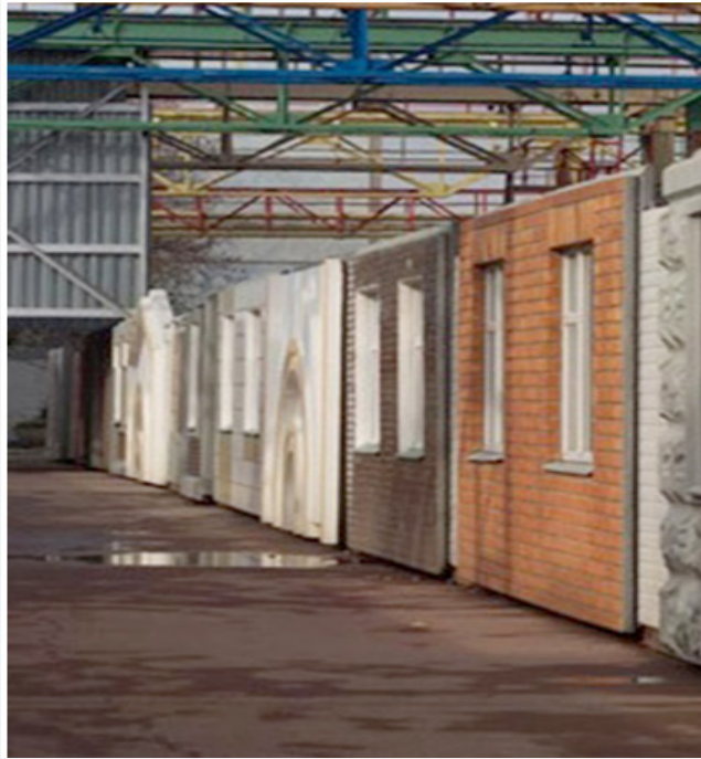
Figure 2: The external wall panels manufactured on new composite nanotechnology at the DSK No. 1 concrete goods Krasnopresnensky plant of Glavmosstroy, 1985. Author of unique ecological nanotechnology of concrete goods chief technologist Alexander Trinker.
