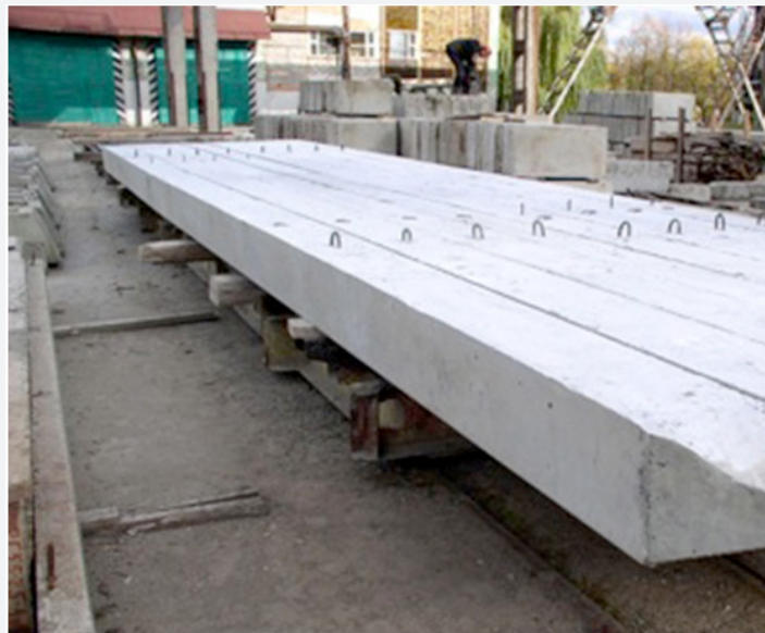
Figure 1: Combined drive piles 17 meters long the Glavmospromstroyaterialy made on new composite nanotechnology at the concrete goods plant No. 17 (Spetsstroybeton), 1985. Author of unique ecological nanotechnology of concrete goods Alexander Trinker.
