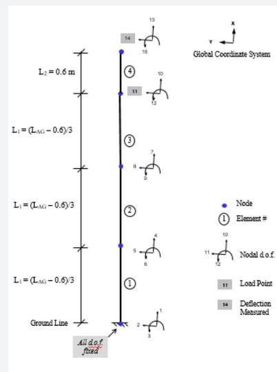
Figure 3: Finite Element Model of System.
