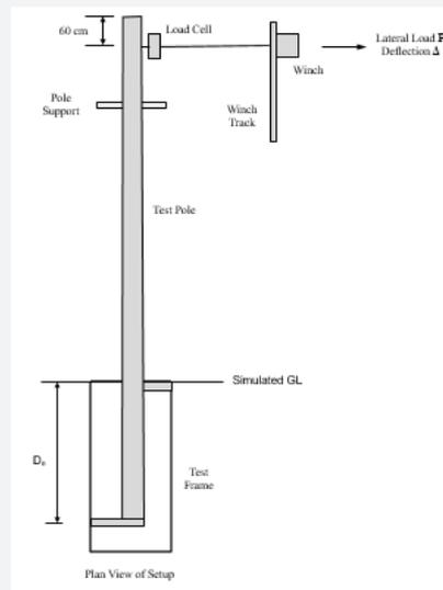
Figure 1a: Test Setup and Instrumentation.
