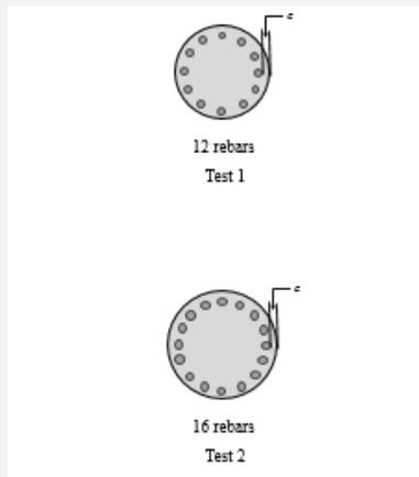
Figure 2: Test Pole Cross Sections Modeled.
