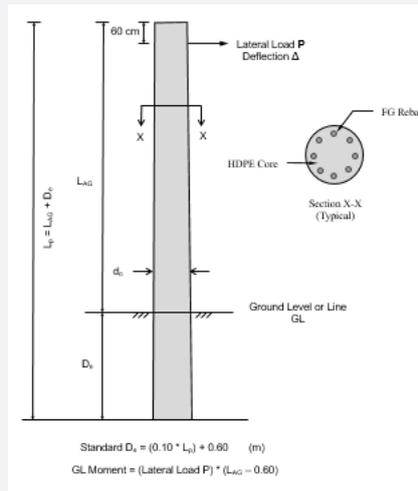
Figure 1: Typical Test Pole and Load Class Definition.
