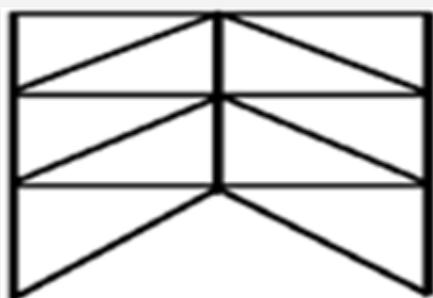
Figure 1: Zipper braced frames.
