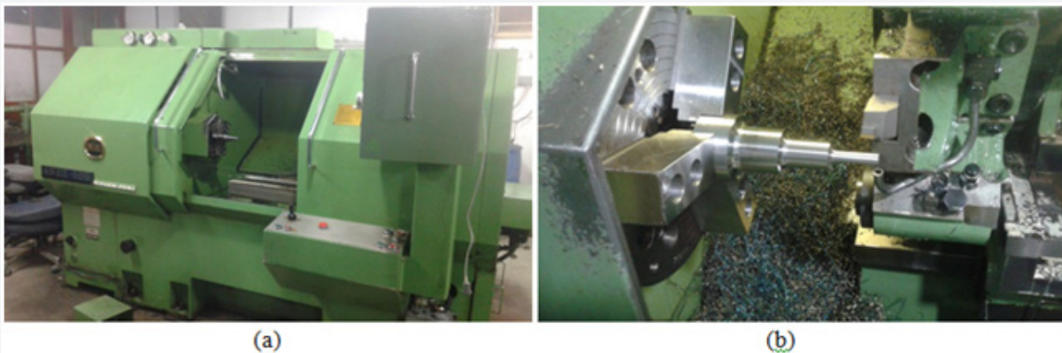
Figure 2: (a) Two axis CNC lathe machine (b) Experimental setup for profile turning.
