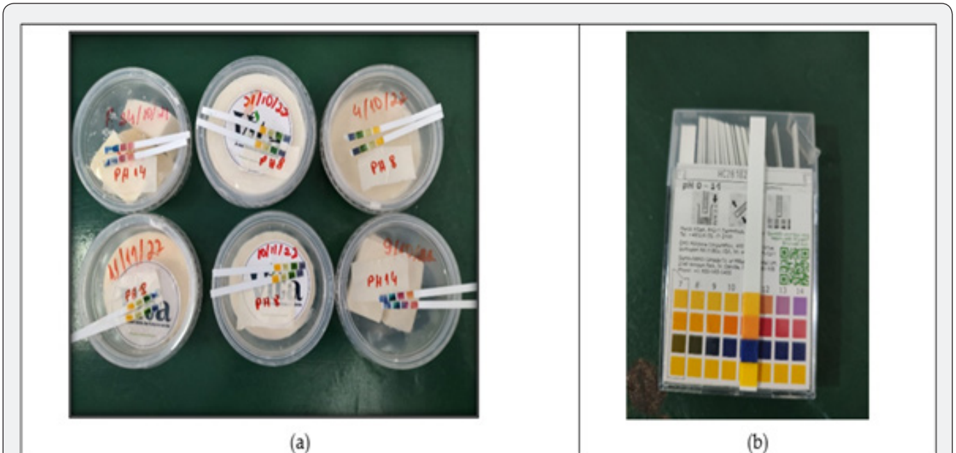
Figure 2: (a) From left to right of the top line are samples with pH 14; pH 8; pH8. And from left to right of the bottom line are samples with pH 8; pH 8 and pH 14. (b) pH titration scale.
