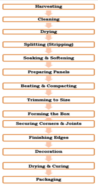
Figure 5: Eco friendly Kora Grass Craft Product design making process.
