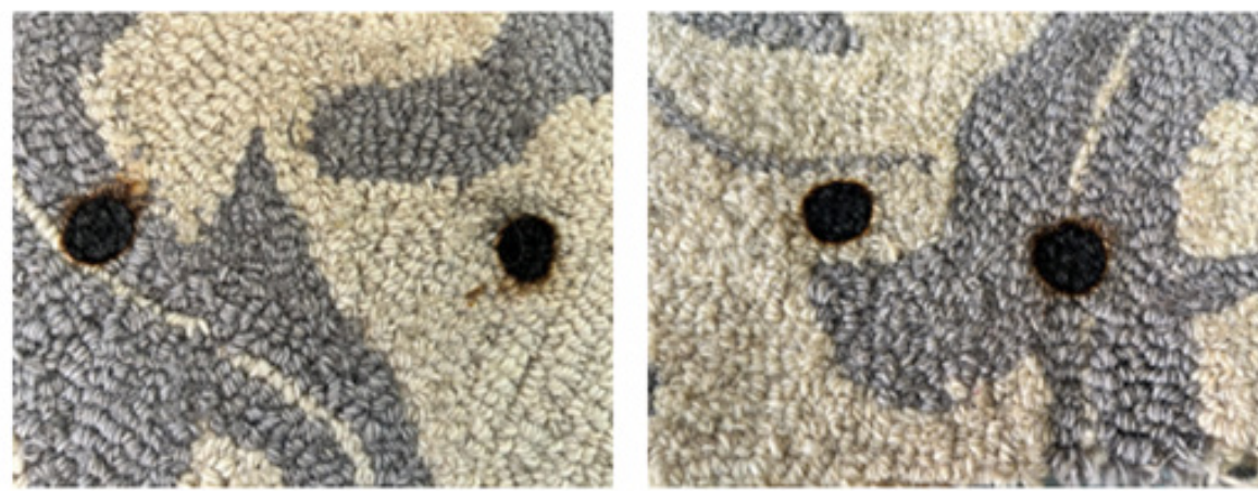
Figure 7: Carpet flammability test with Methenamine tablet test on treated woollenised Jute based carpet.
