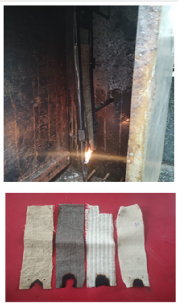
Figure 4: Vertical flame test of Untreated and FR treated woolenised Jute and Jute- Cotton fabrics.
