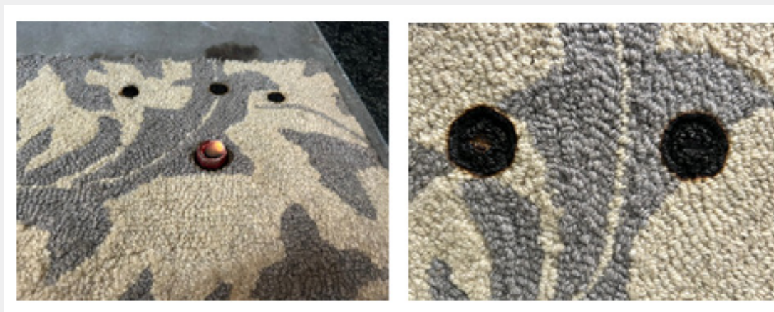
Figure 8: Carpet flammability test with Hot metal nut method on treated woollenised Jute based carpet.
