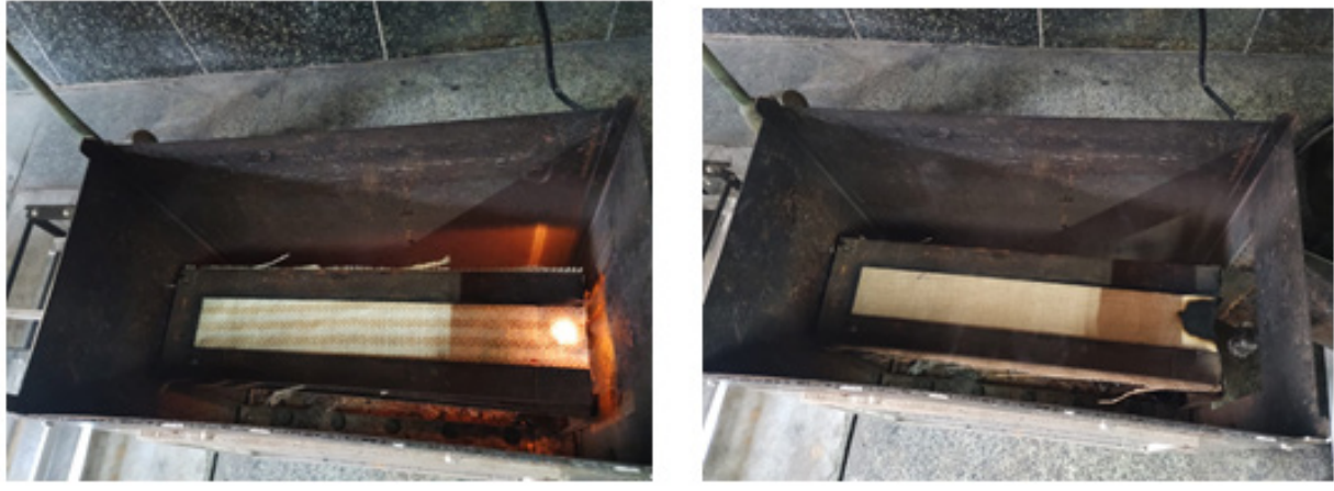
Figure 5: Horizontal flame test of Untreated and FR treated woollenised Jute and Jute- Cotton fabrics.
