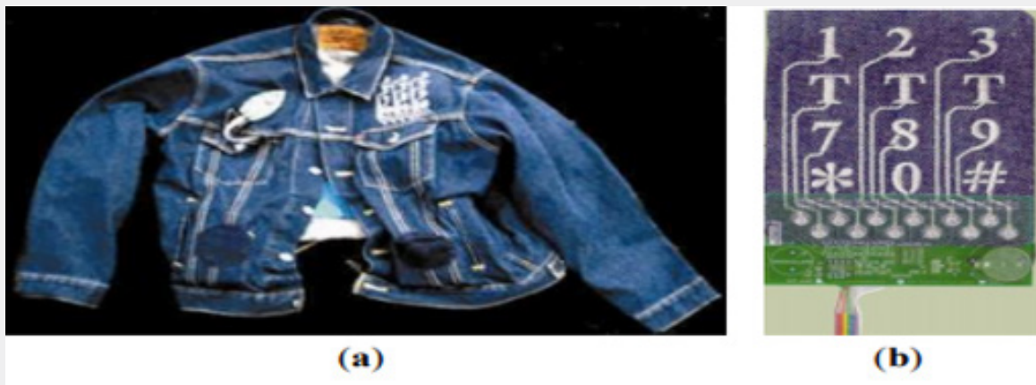
Figure 1: (a) Musical jackets with fabric keypad on one side and (b) fabric keypad (Reproduced with the permission of [2]).
