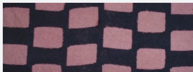
Figure 10: Decrolin Discharged Remazol Black B (8% owf) Dyed Cotton - Diazotisation of Bound Primary Aromatic Amine Followed by H-Acid Coupling.
