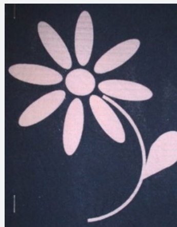
Figure 8: Illuminated Discharge (Single Step Print). Illuminated Discharge Ink Containing Rongalit C and Indigosol Brilliant Pink I5B.
