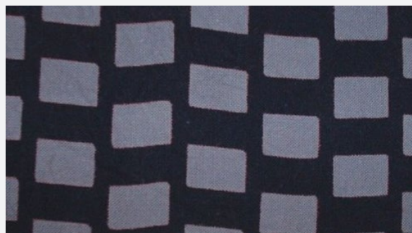
Figure 6: Illuminated Discharge (Single Step Print). Illuminated Discharge Ink Containing Rongalit C and Indigosol Blue IBC.
