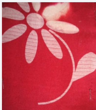
Figure 9: White Discharge on Silk. Decrolin Discharge Ink on CI Acid Red 17 Dyed Silk.
