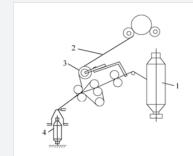
Figure 1: Sirofil spinning process [12].
