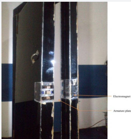
Figure 13: Showing the armature plate and electromagnet when the door is ajar.
