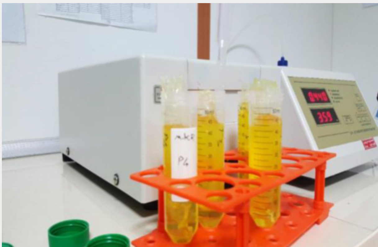
Figure 6: Measuring the light absorption of samples at a wavelength of 359 nm using a spectrophotometer
