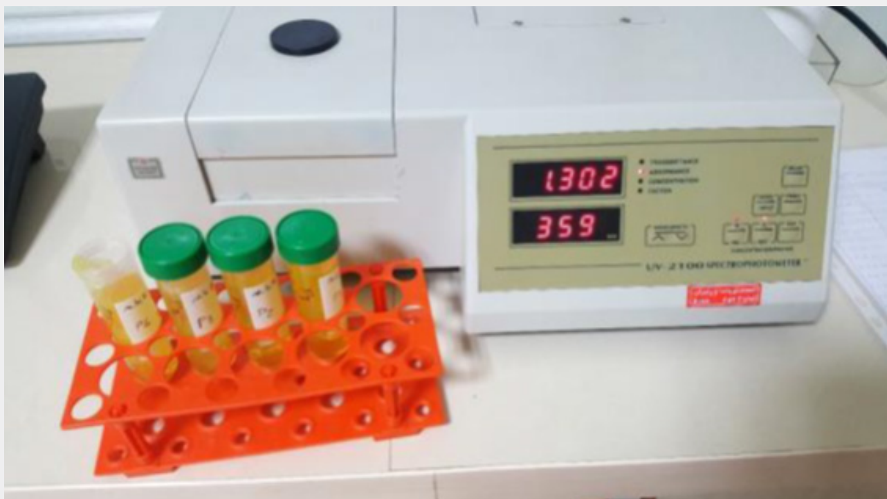
Figure 5: Measuring the light absorption of samples at a wavelength of 359 nm using a spectrophotometer.
