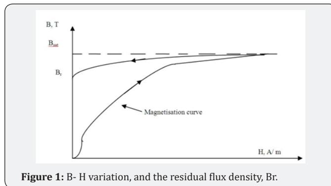
**Figure 1:** B- H variation, and the residual flux density,  $B_r$ .
