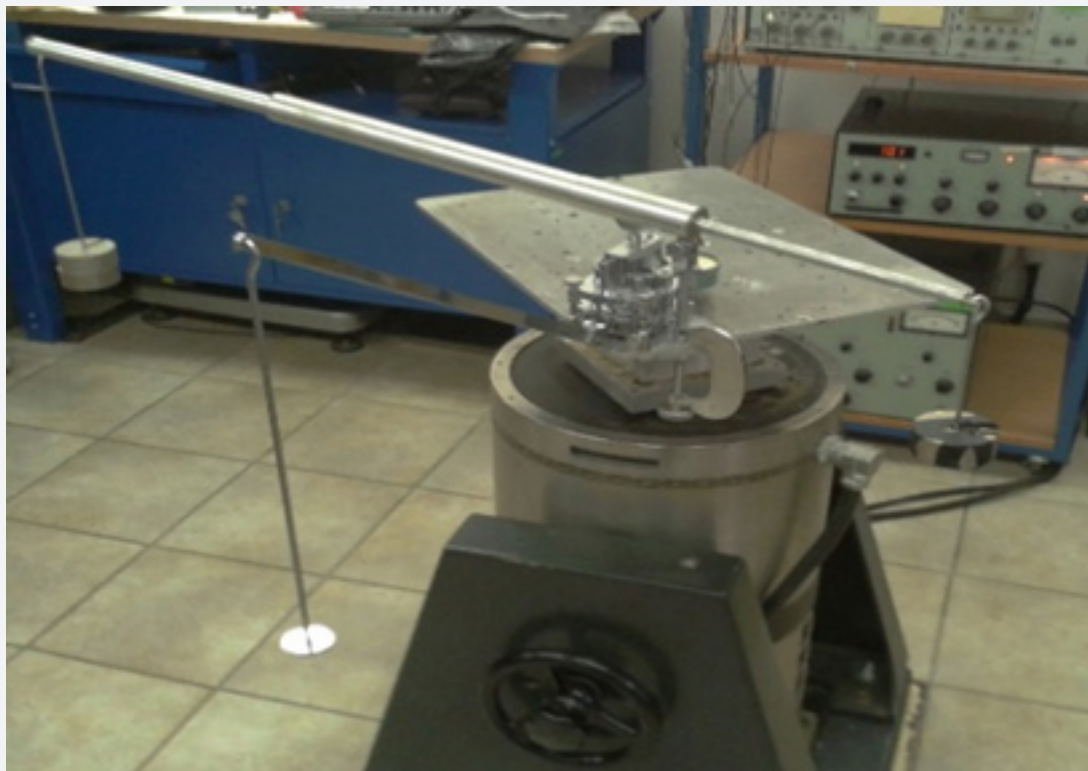
Figure 3: View of shear test using vibrating table (in laboratory of vibration engineering of Kaunas University of Technology).
