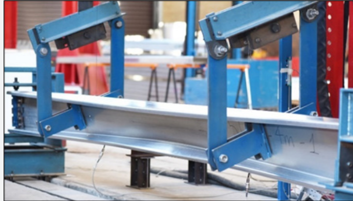
a) Test C25025DL-4.0m-1 (Anti-clockwise failure direction).
