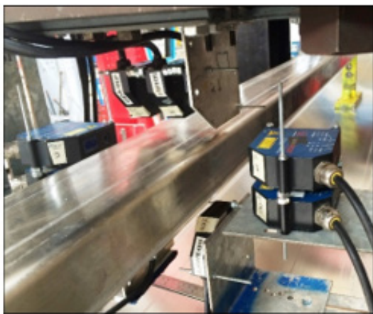
Figure 2: The test rig for measuring geometric imperfections.
