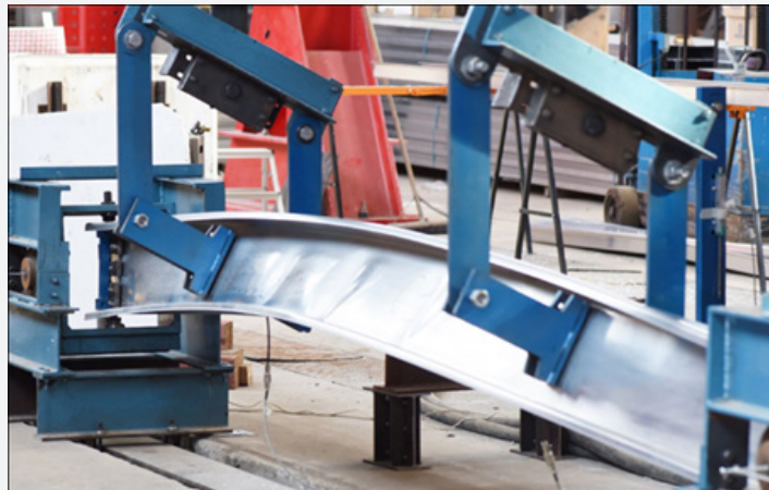
b) Test C25025DL-4.0m-2 (Clockwise failure direction)
