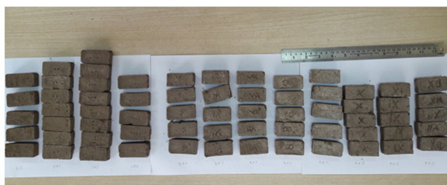
Figure 2: Waste Propellant Impregnated Fire Clay Brick.
