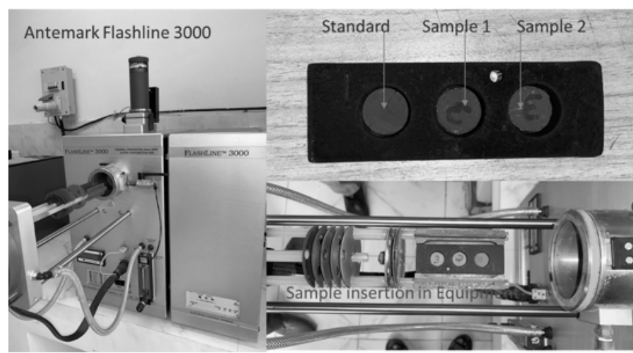
Figure 3: Set-up for Thermal Conductivity Measurement by Laser Flash Method.
