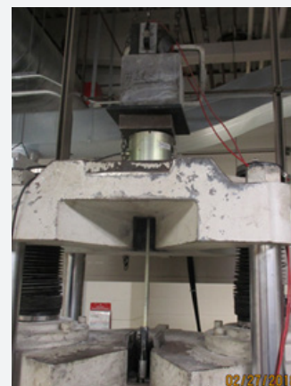
Figure 1: Test setup for a sample 11mm diameter sanded surface specimen.
