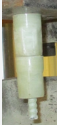
Figure 2: Using two nuts with the threaded surface bar to apply the pullout force by bearing on the nuts.
