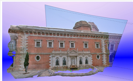
Figure 3: Old University of Valencia. Model with 144 cameras on tripod together with one of the images superimposed.
