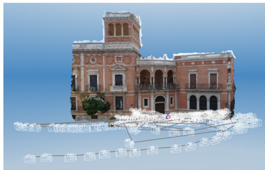
Figure 5: Archbishop's Palace of Valencia Camera tracking in circles to capture on tripod.
