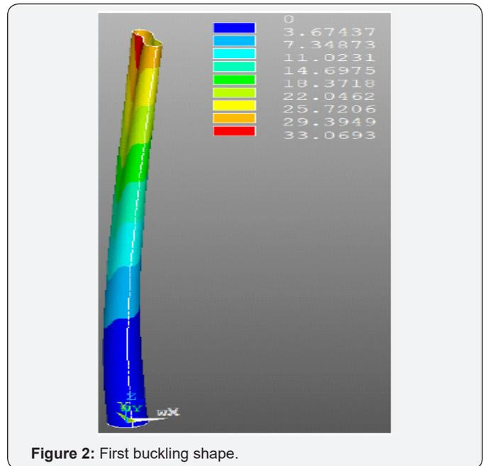
**Figure 2:** First buckling shape.
