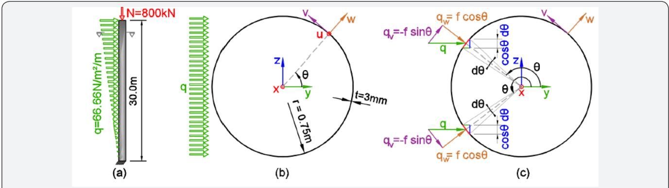
**Figure 1:** Thin-walled circular hollow section under a normal and linear projected force. a) elevation, b) cross section, c) force and projected area in a local coordinate system.
