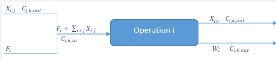
Figure 2: The superstructure model of multi-contaminant-water reuse model
