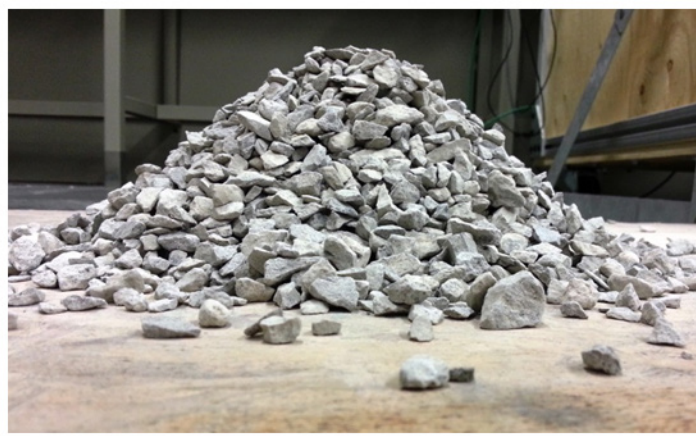
Figure 5: Dolomitic limestone particles piled at 38° angle of repose.
