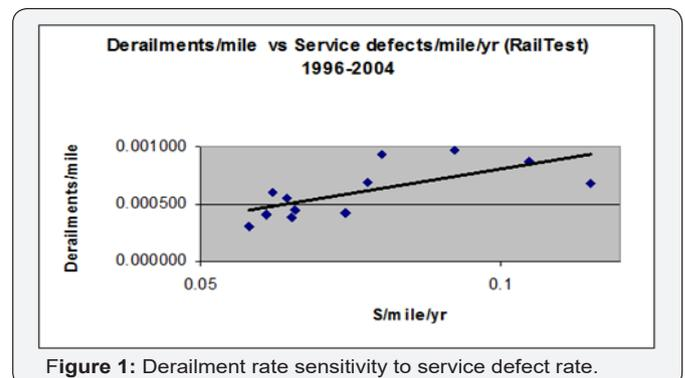
For example, broken rail risk management includes using service defect rate to determine allowable levels of risk (Table 1) and determine ultrasonic rail test schedules. While service defects represent only about 10% of all defects, they have a very strong correlation to derailment occurrence, as shown in Figure 1. Recent studies indicate that a broken rail derailment occurs approximately every 133 service defects for a derailment
