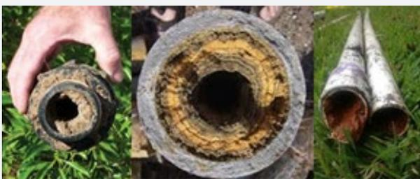
**Figure 1:** Clogging status in different pressurized irrigation systems.
