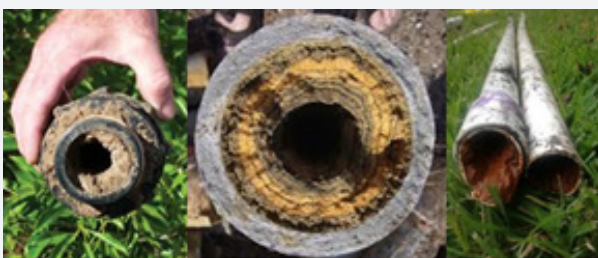
Figure 1: Clogging status in different pressurized irrigation systems.
