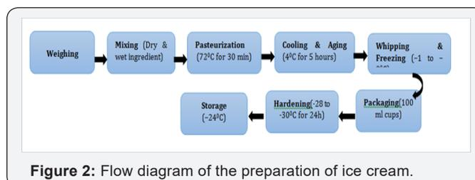
Figure 2: Flow diagram of the preparation of ice cream.
