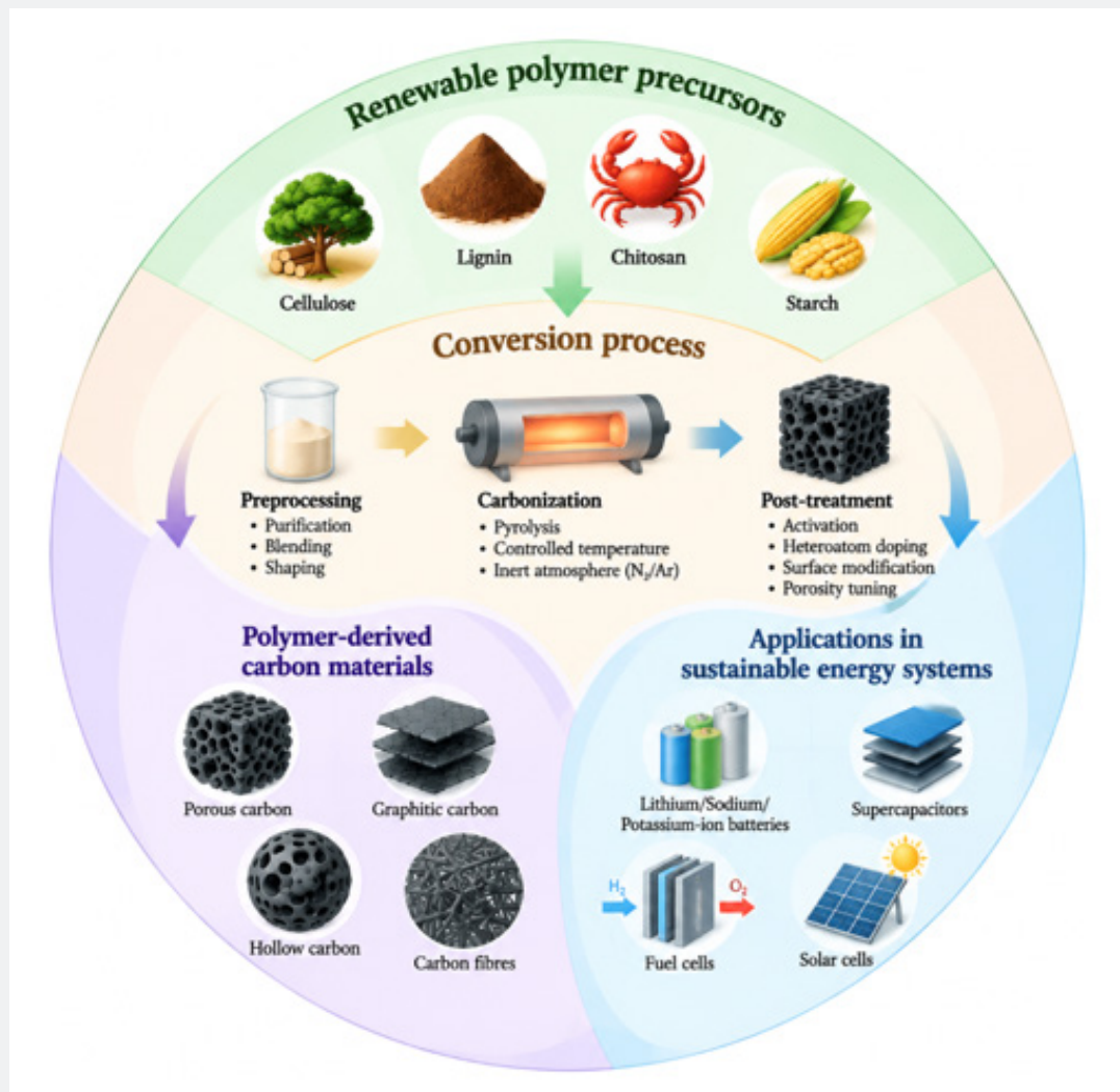
Figure 4: Schematic illustration of polymer-to-carbon conversion pathways and their applications in sustainable energy systems.
