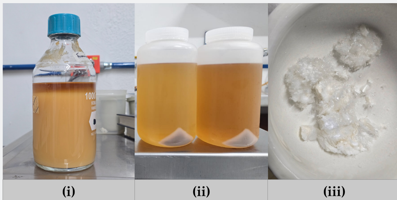
Figure 1: Workflow illustrating the recovery and purification of EPS: (i) 72 h fermentation of L. plantarum LH04, (ii) isopropyl alcohol-induced precipitation, and (iii) purified EPS obtained after dialysis and lyophilization.
