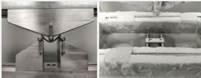
Figure 2: Three-point bending test of T7109-19 epoxy system on RT (left) and T7110 epoxy system on LN2 (right).
