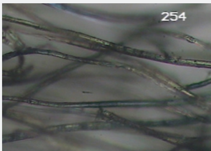
Figure 3: Hydrolysis process (10% HCL, 2h).
