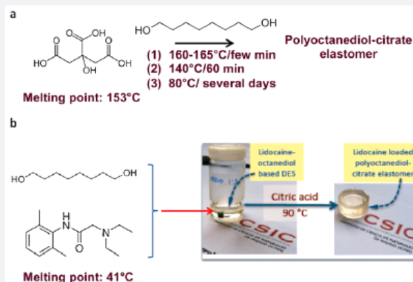
Figure 2: Scheme representing the synthesis of poly(octanediole citrate) from a) 1,8-octanediole dissolved in molten citric acid (at 160°C), and b) a eutectic mixture composed of 1,8-octanediole and lidocaine, the low melting point of which allows the dissolution of citric acid and its subsequent polycondensation at temperatures as low as 90°C. Reproduced with permission from references [7,8].
