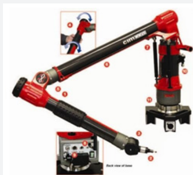
Figure 12: Cimcore brand 3D scanner.
