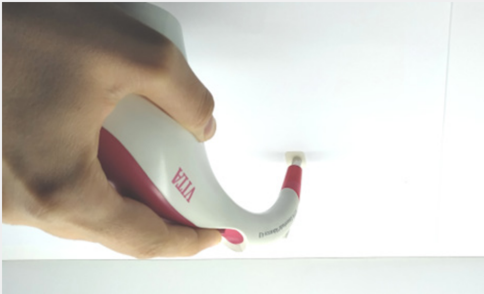
Figure 4: Color measurement using a spectrophotometer device in the special box unit.
