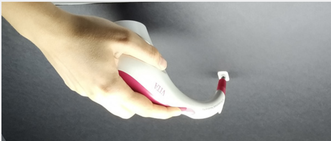
Figure 5: Translucency measurement using a spectrophotometer device in the special box unit.
