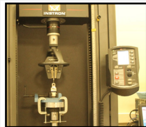
Figure 2: A Specimen loaded in the universal testing machine (Instron).
