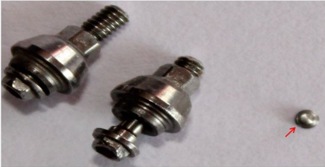
Figure 5: Broken screws retrieved from the multi-unit abutment in 32 and 42 region.
