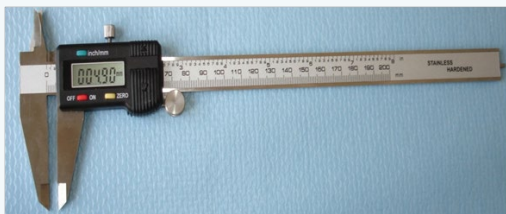
Figure 2: Fowler Electronic Digital Calliper (accuracy was set to \pm 0.1 mm).
