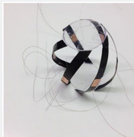
Figure 14b: Actual helically twisted IPMC strips with hinge-hinge ends.
