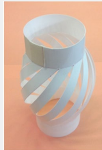
Figure 14a: Possible slit-tubular helical configurations of IPMC strips.
