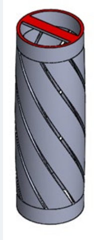
Figure 13a: Helical form of slit IPMC actuators and sensors.
