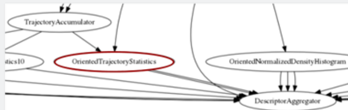
Figure 8.1: The OrientedTrajectory pipeline adds a new statistics node, which is useful for classifying objects with differential vertical and horizontal motion behaviours.
