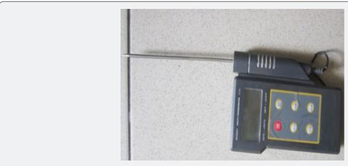
Figure 2: Multi thermometer DT300.
