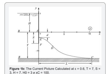
Currents in a rectangular jumper with partially impenetrable vertical wall and to imperfect gallery
