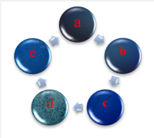
Figure 5: Optical microscope photo (5X) of (a) 75-nm SiN_x by PECVD, (b) 75-nm ZrO_2 by spray deposition, (c) 40-nm of ZrO_2 , (d) 40nm of TiO_2 and (e) photo 40 nm of Ti_{50}-Zr_{50} oxide by dc-pulsed Magnetron Sputtering.
