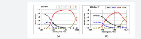
Figure 2: Structures diagrams of steels 20CrNi4V (a) and 25Cr2Mo1V (b) depending on the cooling rate (F - ferrite P - pearlite; B - bainite; M - martensite).
