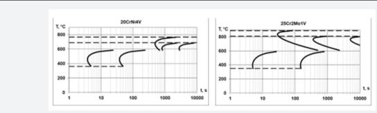
Figure 1: TTT diagrams of alloy steels.
