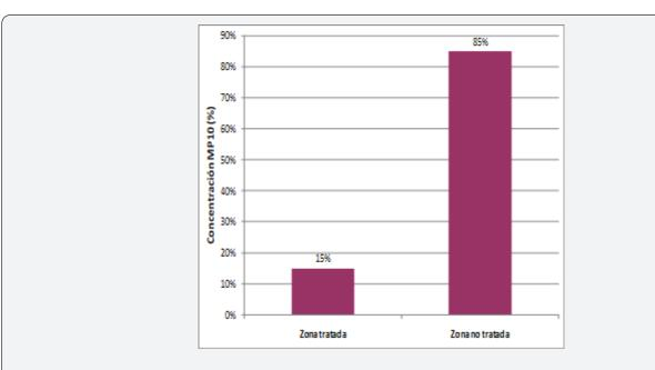
Figure 5: Distribution of total PM10 registered, according to location in treated and untreated areas, tailings dam.
