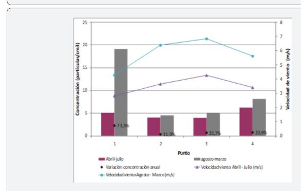
Figure 6: Averages of wind speed and concentration of PM10 and its variation in monitoring stations.
