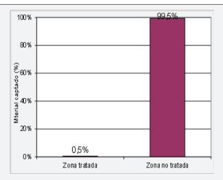
Figure 3: Distribution of the total material captured in the Leatherman traps, according to its location in the area treated with dust suppressant and untreated areas.
