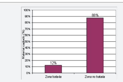
Figure 4: Distribution of the total material collected in the dust collectors, location in the area treated with dust suppressant and untreated areas.
