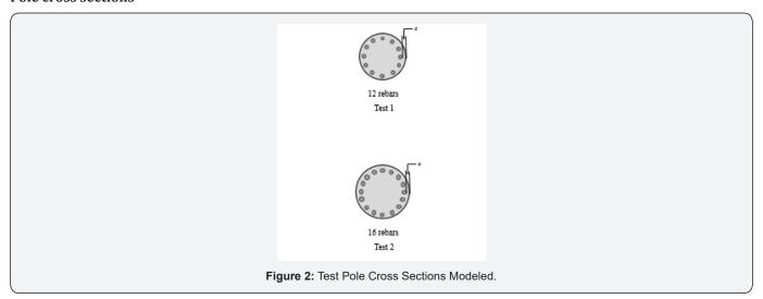
Figure 2 shows pole cross sections associated with different test configurations of rebars. Two (2) cross sections with 12 and
