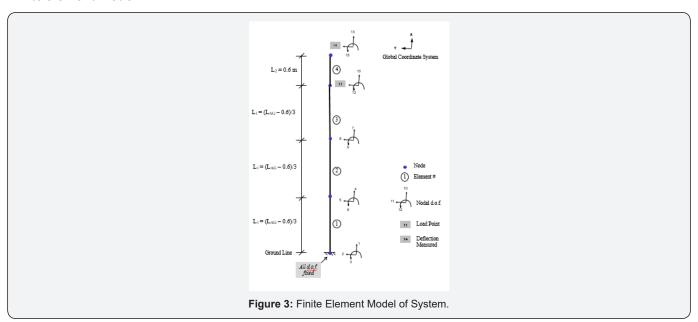
As shown in Figure 3, the pole system is modeled with four (4) planar beam elements each with 6-d.o.f. (degrees of freedom), with a top element  $L_2$  of 60cm (2 feet) length consistent with the definition of pole class. The bottom three elements are of equal length  $L_1$ .
