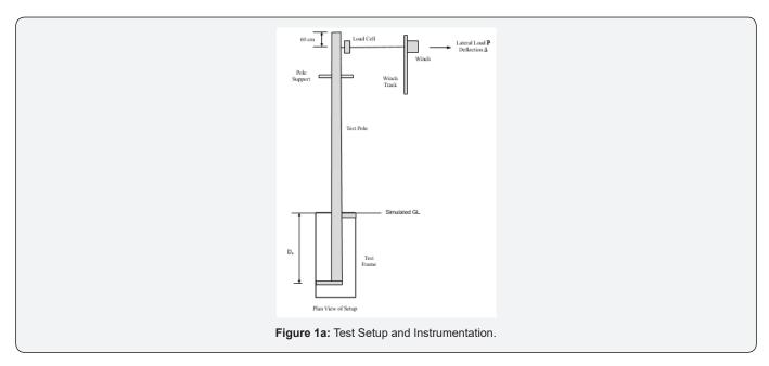
The poles were tested as a **cantilever** with a single lateral load; deflection measurements were made at each load step [5]. The loading is applied at a constant rate and deflection was measured primarily at the pole tip from which deflection at load point was deduced. Both poles were tested until complete failure which is
