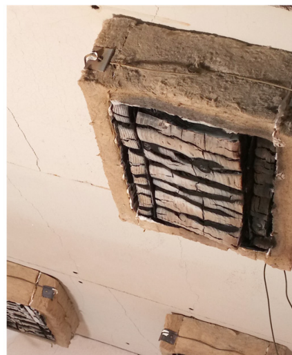
Figure 11: Charred layer on the samples after the end of the test.
