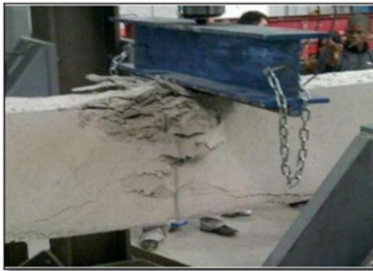
Figure 5: Some of the examples of concrete failures. The photo on the left-hand side is a flexural compression failure and the right one indicates a shear failure. [14].
