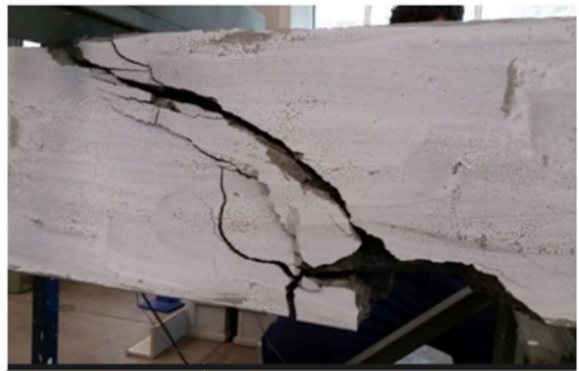
Figure 5: Some of the examples of concrete failures. The photo on the left-hand side is a flexural compression failure and the right one indicates a shear failure. [14].
