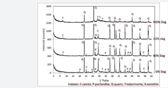
Figure 6: X-ray diffraction patterns of synthesis products at saturated vapour pressure of 1.8MPa (204 °C).
