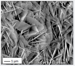
Figure 4: SEM micrograph of 11Å tobermorite morphology
