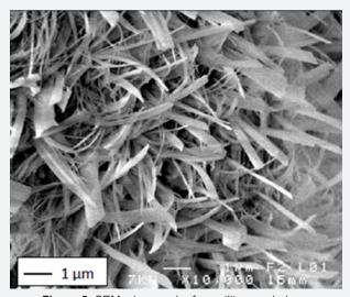
Figure 5: SEM micrograph of xonotlite morphology.
