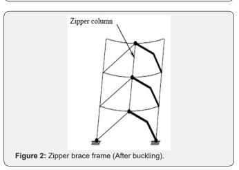
With a proper zipper configuration, it is possible to address the problems and weaknesses of the chevron bracing frame [11].
