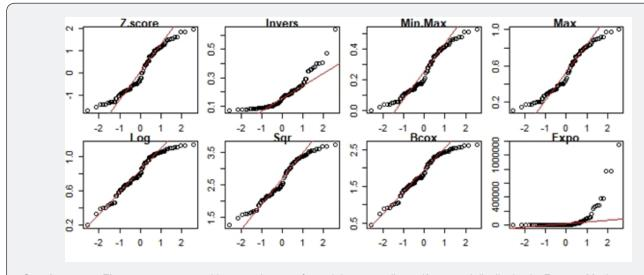
**Supplementary Figure 4:** qqnorm graphic assessing transformed data normality and/or normal distribution by Z-score, Maximum, Maximum-Minimum, Square root, Inverse, Logarithm and Box-Cox data transformation procedures
