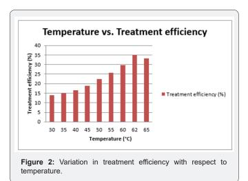
Involvement of thermopiles in the experiment confirms the obvious supply of external heating system which has been compensated by a 60 W electronic bulb. It worked as a dual source of light and heating at the same time and the temperature in the heap often found to reach a threshold value of 62 °C [20]. Two major parameters of interest namely, treatment efficiency and temperature portrayed a proportional relationship within a temperature range of 30 °C to 65 °C though, any further
